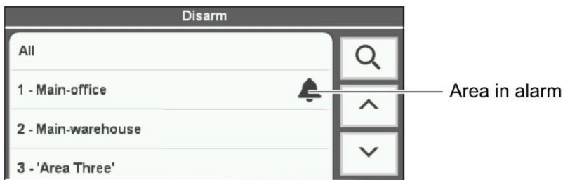
Figure 9: Disarm screen showing area in alarm
