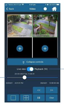
Live view / Playback – Toggles the video between live video and recorded video. When Playback is selected, this toggle also shows the current playback speed.
