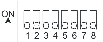
Figure 3: DIP switches for LAN addressing and termination
