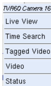
Figure 22: LAP menu for a Challenger device programmed with an associated video camera
